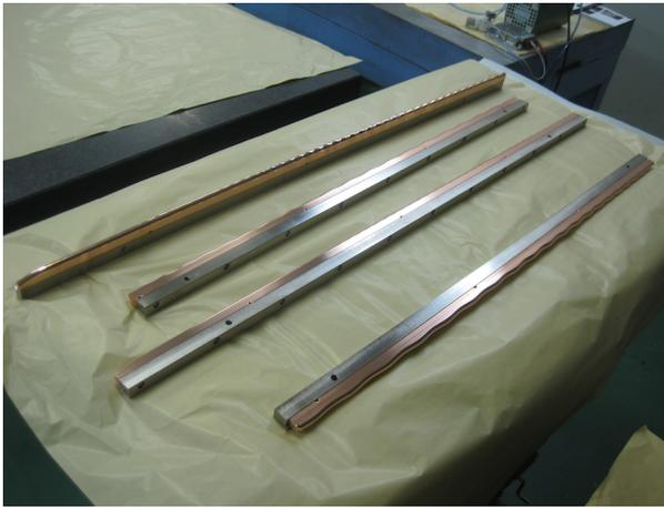
Figure 3: The manufactured RFQ electrodes.
