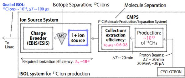
Figure 2: A scheme to provide <sup>11</sup>C ion beam (borrowed from Ref. [8]).
