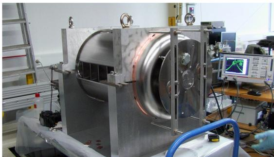
Figure 5: The first sc CH-cavity during manufacturing.
