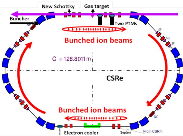
Figure 8: Layout of laser cooling at CSRe.
