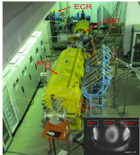
Figure 6: SSC-Linac testing platform.
