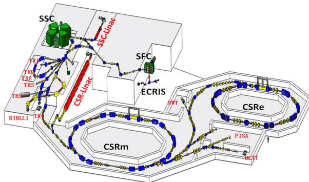
Figure 4: Layout of HRFL with new injectors.
