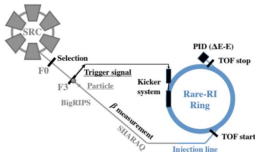
Figure 1: Conceptual design of mass measurement with the Rare-RI Ring located after the SHARQA spectrometer.
