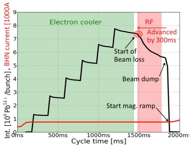
Figure 4: LEIR ion beam intensity with advanced RF-capture and main bending magnet current versus cycle time.
