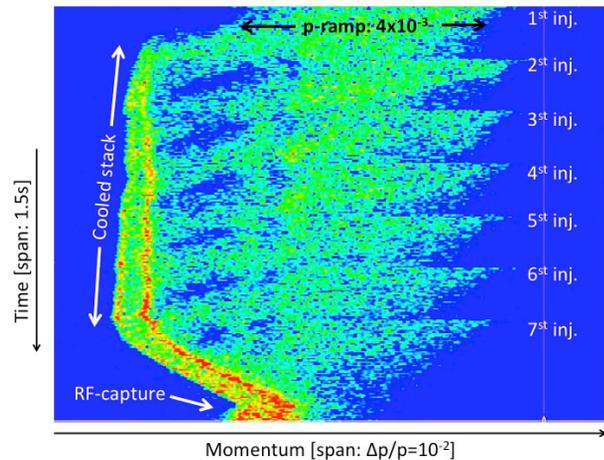
Figure 5: Schottky spectrum in momentum space of the  $Pb^{54+}$  ion beam in LEIR in a waterfall diagram (time versus beam momentum).
