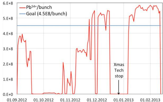
Figure 2: Extracted ions per bunch from LEIR from September 1<sup>st</sup> 2012 until February 1<sup>st</sup> 2013. The intensity goal of the LHC ion run for LEIR was 4.5x10<sup>8</sup> ions per bunch, which was achieved in January 2013.
