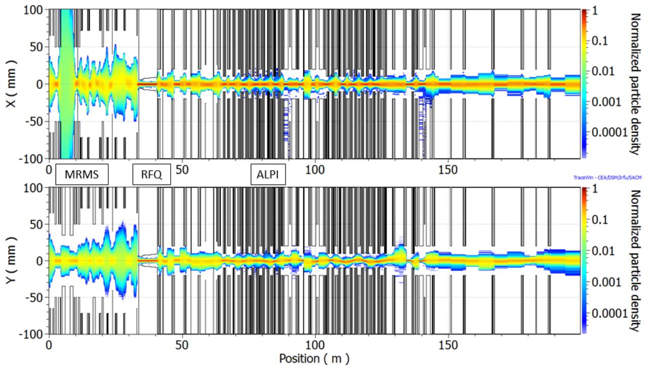
Figure 4: Multiparticle normalised-densities y and x of the whole line CB-RFQ-ALPI- Experimental hall.
