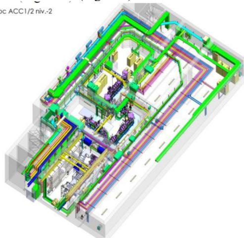
Figure 4: 3D views of processes + connections + buildings.
