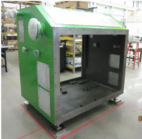
Figure 7: Photo of the secondary containment vessel installed in the test area of FRIB. The vessel is 2 m long.
