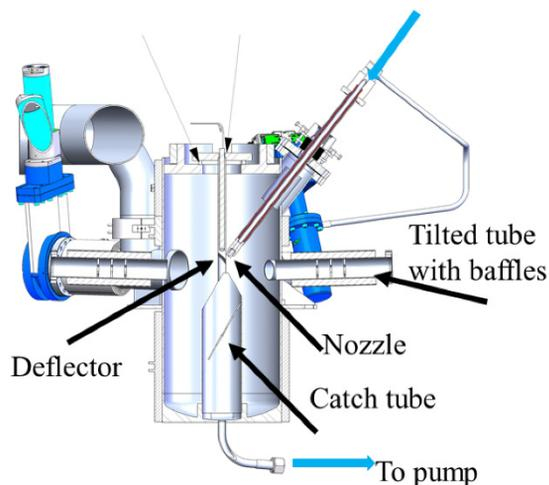
Figure 5: Main vacuum chamber showing the incoming lithium on the upper right and the exit to the pump in the lower right.
