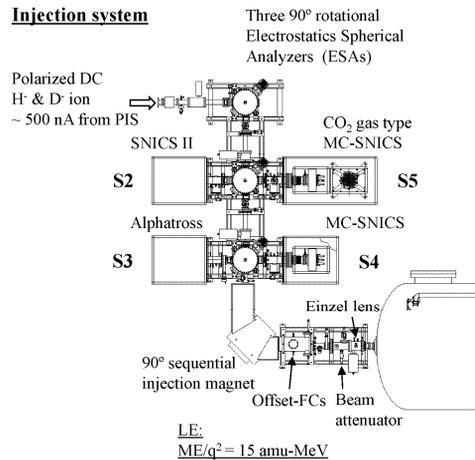
Figure 3: Injection system of the 6 MV tandem accelerator.
