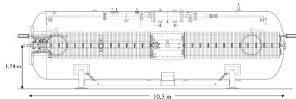
Figure 4: Cross-section drawing of the accelerator tank.
