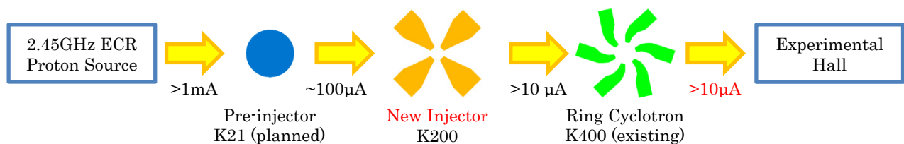
Figure 2: One example of proton acceleration in current RCNP cyclotron cascade.
