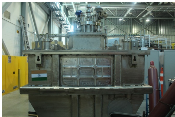
Figure 5: Injector Cryo Module for the VECC superconducting Electron Linac (e-Linac) at TRIUMF.
