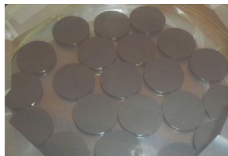
Figure 3: Photograph of 1-mm uranium-oxide-coated target disks. These disks are 20 mm in a diameter and 1 mm in a thickness.
