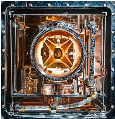
Figure 3: View along the ion beam path into a cryogenic quadrupole unit of the CSR. The electrodes in the center are surrounded by the cryogenic vacuum chamber, refrigerant tubes, and two radiation shields with the inner one serving as a mechanical chassis held at 40 K.
