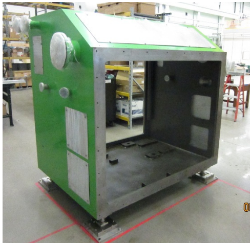
Figure 7: Photo of the secondary containment vessel installed in the test area of FRIB. The vessel is 2 m long.
