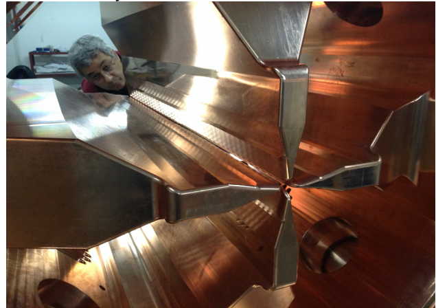
Figure 7: First segment of the RFQ at the vendor site.
