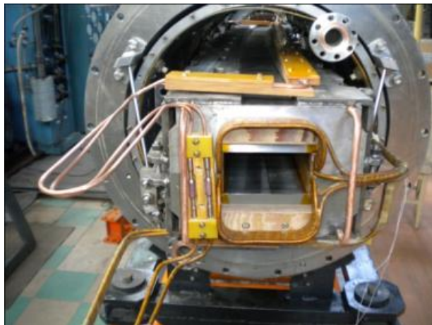
Figure 5: Pre-serial dipole magnet of the NICA Booster.
