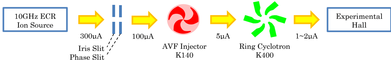
Figure 1: One example of proton acceleration in current RCNP cyclotron cascade.
