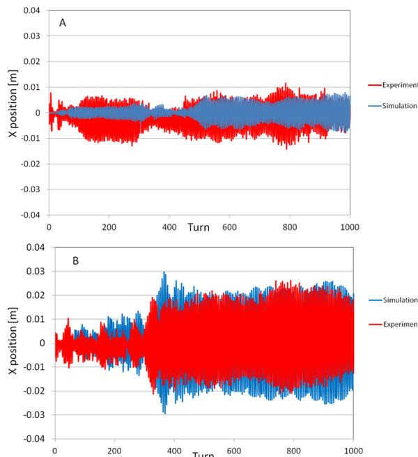
Figure 7: Simulation (blue) and experimental (red) results of temporal evolution of the beam centroid for Plan A and Plan B.
