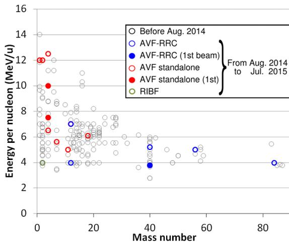
Figure 2: Energy per nucleon versus mass number of ions extracted from the AVF cyclotron.
