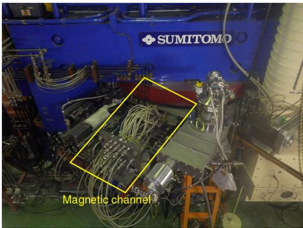
Figure 5: Magnetic channel of the AVF cyclotron.
