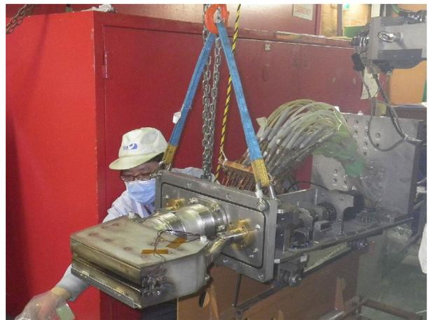
Figure 8: A new magnetic channel.
