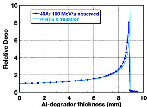
Figure 4: Depth-dose curves for a 160-MeV/nucleon argon beam.
