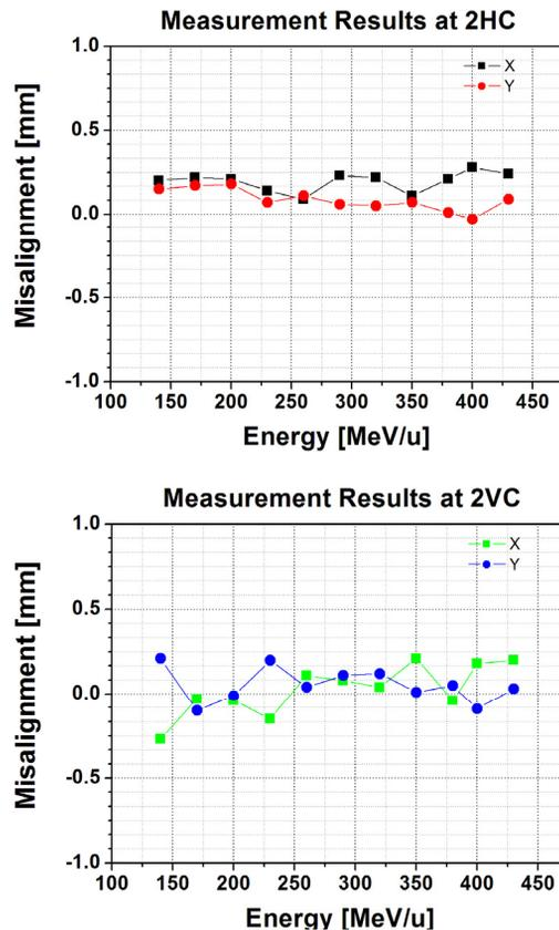
Figure 6: Measurement results of the beam misalignment.
