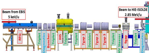
Figure 9: Layout of REX normal conducting post-accelerator.
