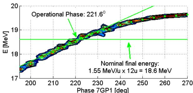
Figure 13: Phasing of the first 7gap RF structure using a silicon detector.
