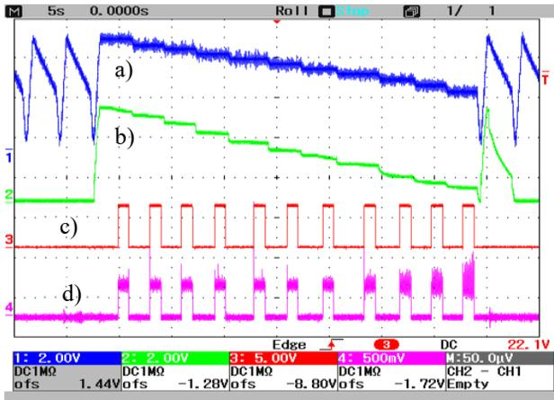
Figure 3: Spill in one cycle with the flat-top extension operation (all 11 energy). a) BM current, b) DCCT, c) Enable signal of extraction and d) Dose monitor.
