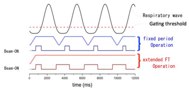
Figure 2: Schematic picture of an extended flat-top operation.
