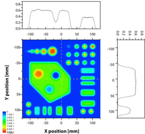
Figure 7: Measurement result with the comprehensive pattern (2 mm pitch, 290 MeV/u).
