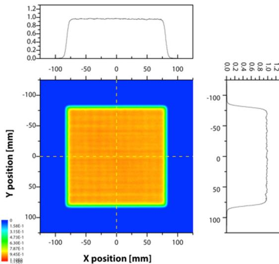
Figure 6: Measured distribution of the uniform field (150 x 150 mm<sup>2</sup>, 2 mm pitch, 290 MeV/u).
