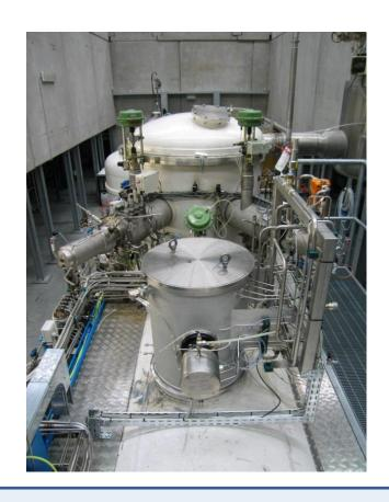
**2012**: **3**<sup>rd</sup> **supercritical turbine** in place of WE, to increase refrigeration capacity at 4,5K **with the JT** expansion valve
