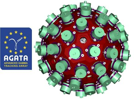
The innovative use of detectors in position-sensitive mode (combining digital DAQ, pulse shape analysis,  $\gamma$ -ray tracking) will result in high efficiency (~40%) and excellent energy resolution, making AGATA the ideal device for spectroscopic studies of weak channels.
