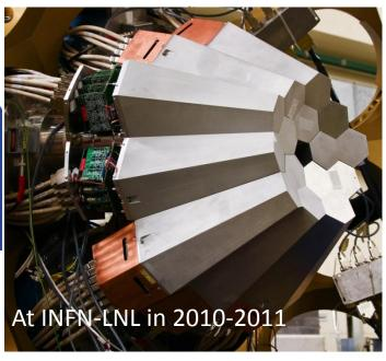
The innovative use of detectors in position-sensitive mode (combining digital DAQ, pulse shape analysis,  $\gamma$ -ray tracking) will result in high efficiency (~40%) and excellent energy resolution, making AGATA the ideal device for spectroscopic studies of weak channels.
