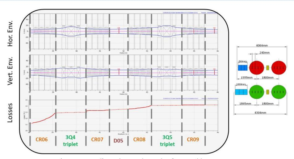
Losses (37% in total) are located on the first and last cavities, in a row of 8 with no quads in between
