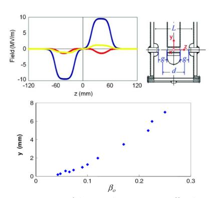
Correction of the QWR beam steering effect by offset beam axis
