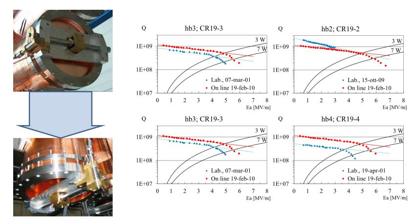
Removal of the In gasket, replaced by a high pressure gasket-less joint is beneficial to the Q, removing a source of dissipation.
