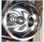
Rounded-off shorting plate & beam ports, **E**<sub>a</sub>~**5,5 MV/m**
