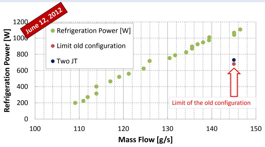
Measured increase in the refrigeration capacity 360 W (predicted 300W): +51%
