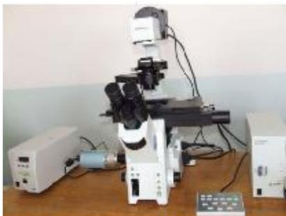
Inverted microscope for cell irradiation
