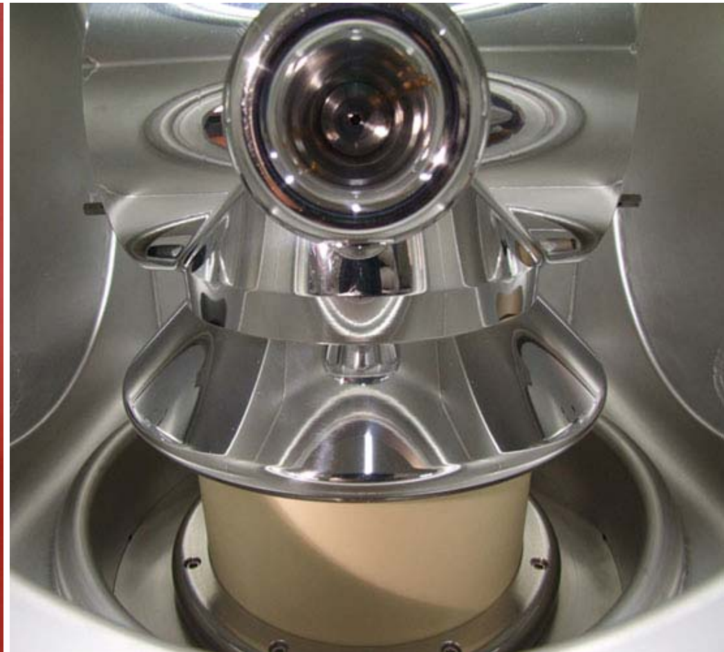
200 kV corona gap inside acceleration unit
