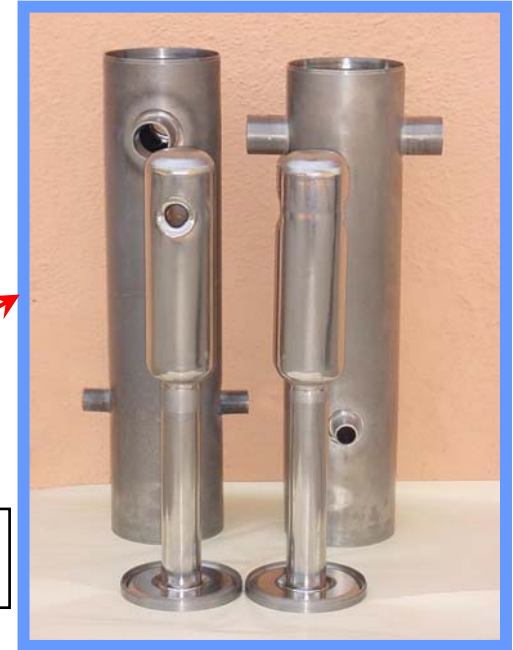
Central conductor and housing
