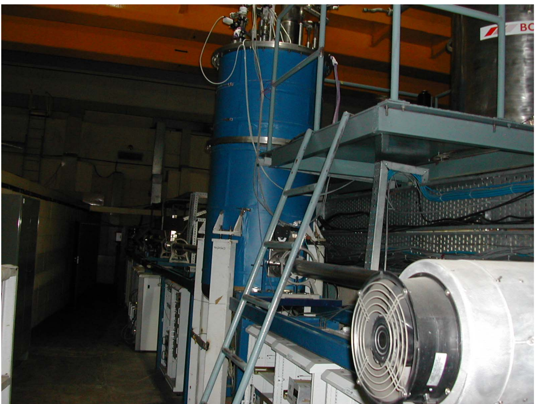
Superbuncher in the beam line (FWHM~170 ps)
