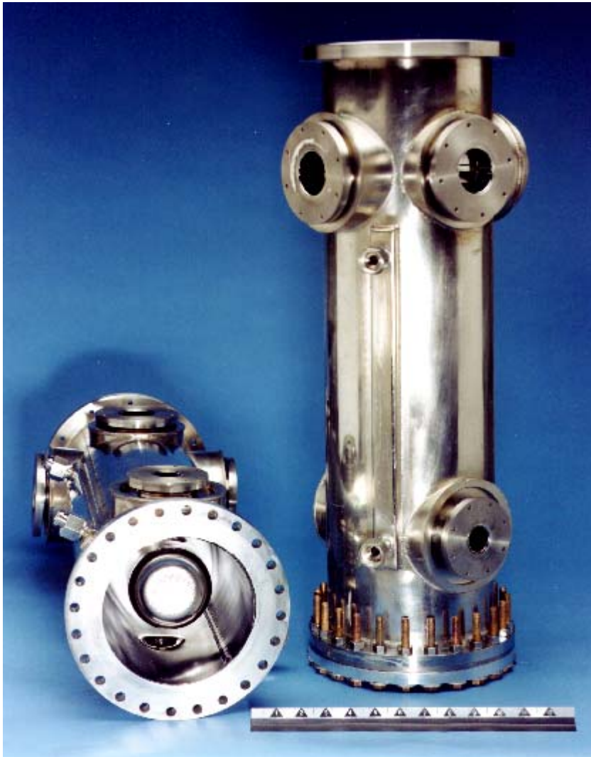
IUAC Quarter Wave Resonator (QWR)
