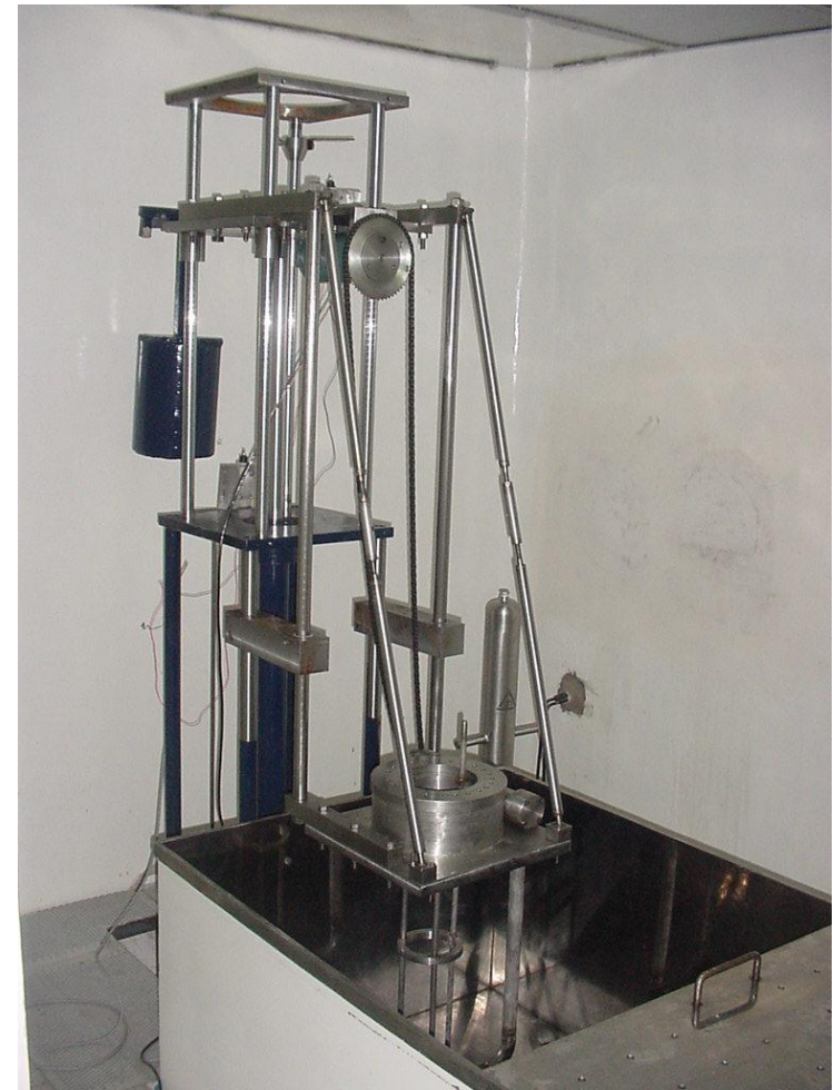
High Pressure rinsing system
