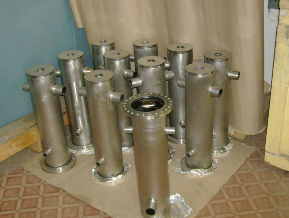
Bare niobium QWRs ready for the outer stainless steel jacketing
