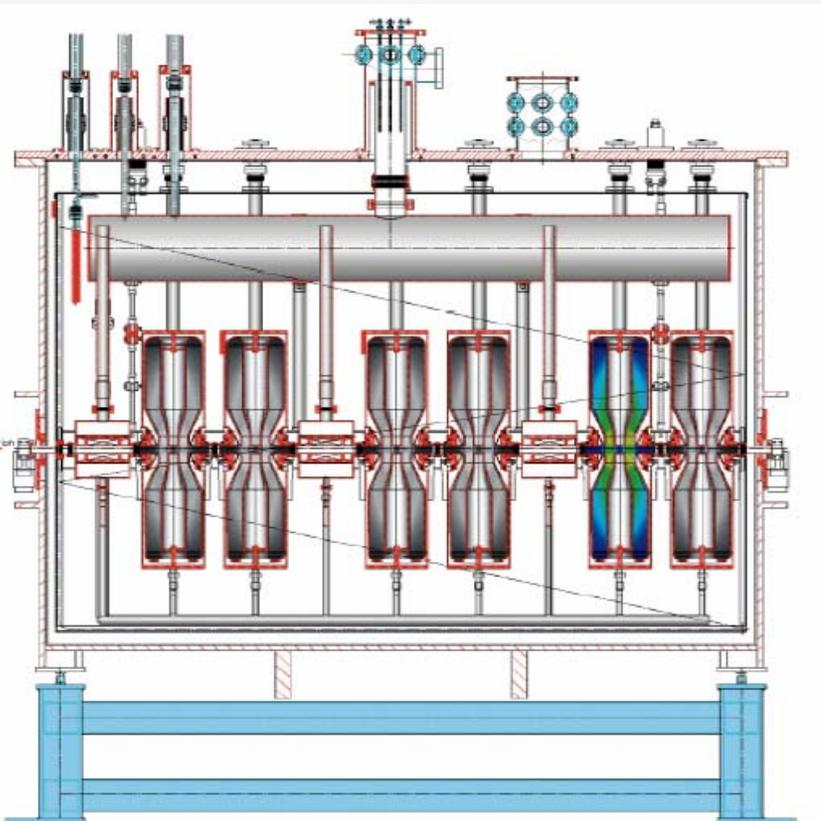
Prototype superconducting module with separate cavity and cryogenic vacuum. Fabrication by ACCEL
