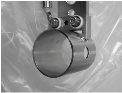
Figure 9: PAT (Post Acceleration Tube) for observation of momentum spread of the laser cooled Mg ion beam.
