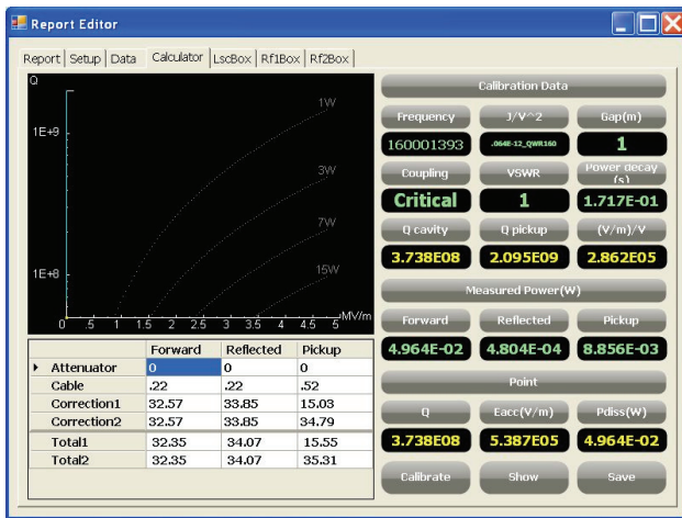
Figure 4. Options Window with RF Calculator panel.
