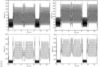
Figure 13: Optics (left:  $\beta_x$ , right:  $\beta_y$ ) with 100 (top) and 300-m (bottom) arc cell length for operation at the *W*-pair threshold (80 GeV) and *Z* pole (45.5 GeV energy) [27].
