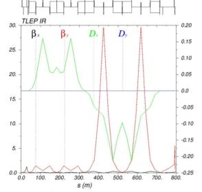
Figure 17: First modular IR design with dedicated chromatic correction sections [32]
