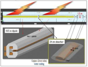
Figure 15: FLUKA geometry layout for half a FODO cell, showing dipole details with a preliminary absorber design including a 5-cm external *Pb* shield [31].
