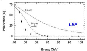
Figure 29: LEP polarization as a function of beam energy. Data points show the measured values. Solid and dashed 2 lines correspond to model predictions [45].
