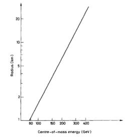
Figure 3: Cost-optimized circumference of a circular  $e^+e^-$  collider versus centre-of-mass energy as of 1976 [3].
