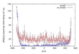
Figure 16: Simulated longitudinal peak-dose profile without (red) and with absorbers (blue) after operating with 10 mA beam current at 175 GeV over a time of  $10^7$  s (116 days, or one "Snowmass year") [31].
