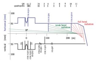
Figure 20: LEP IR design with weak bend and multiple masks [36].
