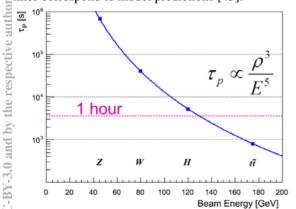
Figure 30: *FCC-ee* natural polarization time versus beam genergy [29].
