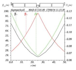
Figure 9: Arc-cell optics at 120 and 175 GeV [27].
