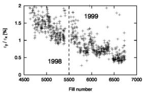
Figure 2: Vertical-to-horizontal emittance ratio at LEP in 1998 and 1999 [1]. The decrease reflects both changes in the damping partition numbers and improved steering [2].
