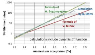
Figure 23: Beamstrahlung lifetime for *FCC-ee* at 350 GeV c.m. as a function of momentum acceptance  $\eta$ , comparing analytical expressions by V. Telnov [41] (red) and A. Bogomyagkov [24] (green) with simulation results from K. Ohmi (blue) [43]. The analytical calculations include the dynamic beta functions matching the simulations.
