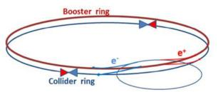
Figure 28: Schematic of booster and collider rings for fast top-up injection [4].
