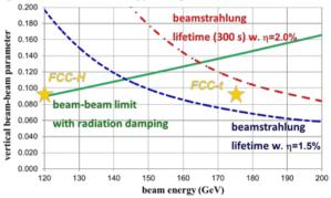
Figure 22: Limits due to classical beam-beam effect and due to beamstrahlung, with two different values for the energy acceptance, as a function of beam energy [42].
