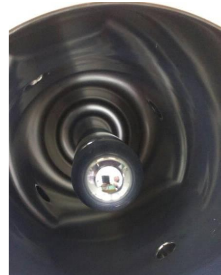
The QWR cavity before and after the sputtering process
