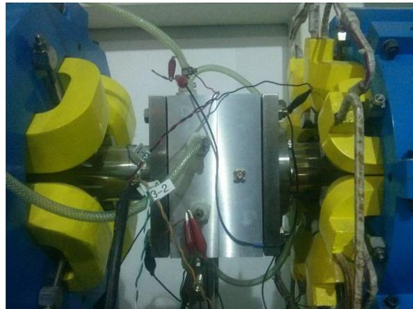
Figure 15: The button-type BPM on the beam line.
