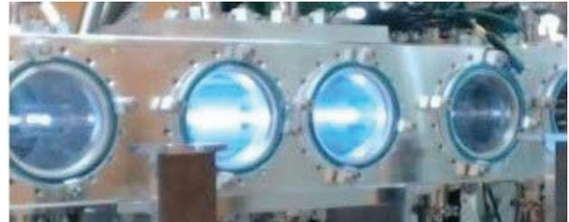
Figure 5: Test of He gas charge stripper using Uranium beams at RIKEN [39].
