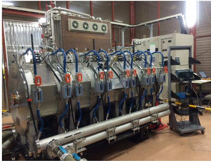
Figure 2: The FT3L cavity during high power test. The cavity consists of 5 cells. Each cell connected to two common bus bars driven by a tube amplifier behind the cavity. The total RF voltage of 80 kV was generated during the high power test in the summer and fall. In total, the cavity system was tested for more than 1000 hours.
