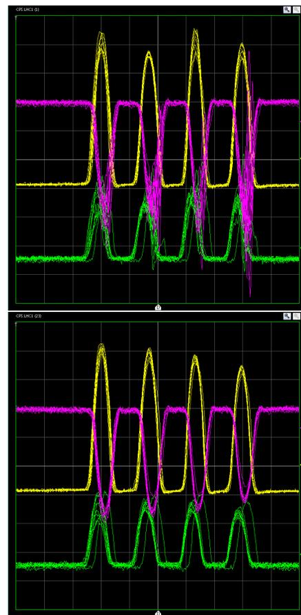
Figure 3: LHC-type bunches injection oscillation without (*top*) and with (*bottom*) the TFB.  $\Sigma$  (yellow),  $\Delta H$  (green),  $\Delta V$  (magenta) (200 ns/div, 200 mV/div). On the plots 50 consecutive turns of 4 LHC-type bunches in the PS are overlapped.
