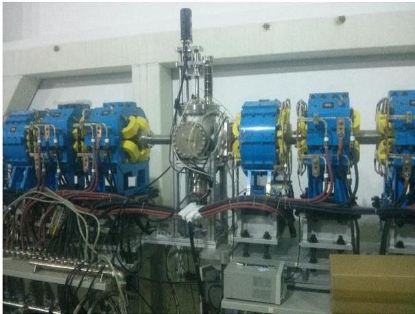
Figure 10: 2D beam profile measurement system.
