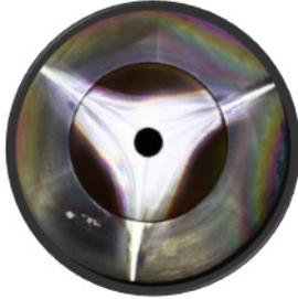
Figure 8: Plasma bombardment images on plasma electrode.
