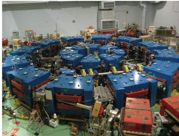
Figure 1: The KURRI 150 MeV FFAG is the larger ring shown here with the pre-2011 injector ring. Injection from the new linac occurs in the top left of the image.
