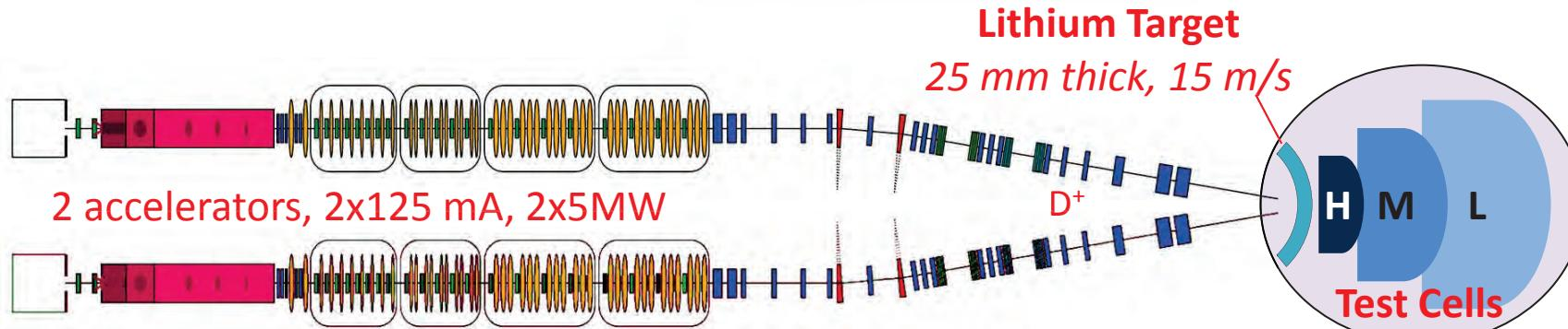
Typical reactions  ${}^7\text{Li}(\text{D},2\text{n}){}^7\text{Be}$   ${}^6\text{Li}(\text{D},\text{n}){}^7\text{Be}$   ${}^6\text{Li}(\text{n,T}){}^4\text{He}$
