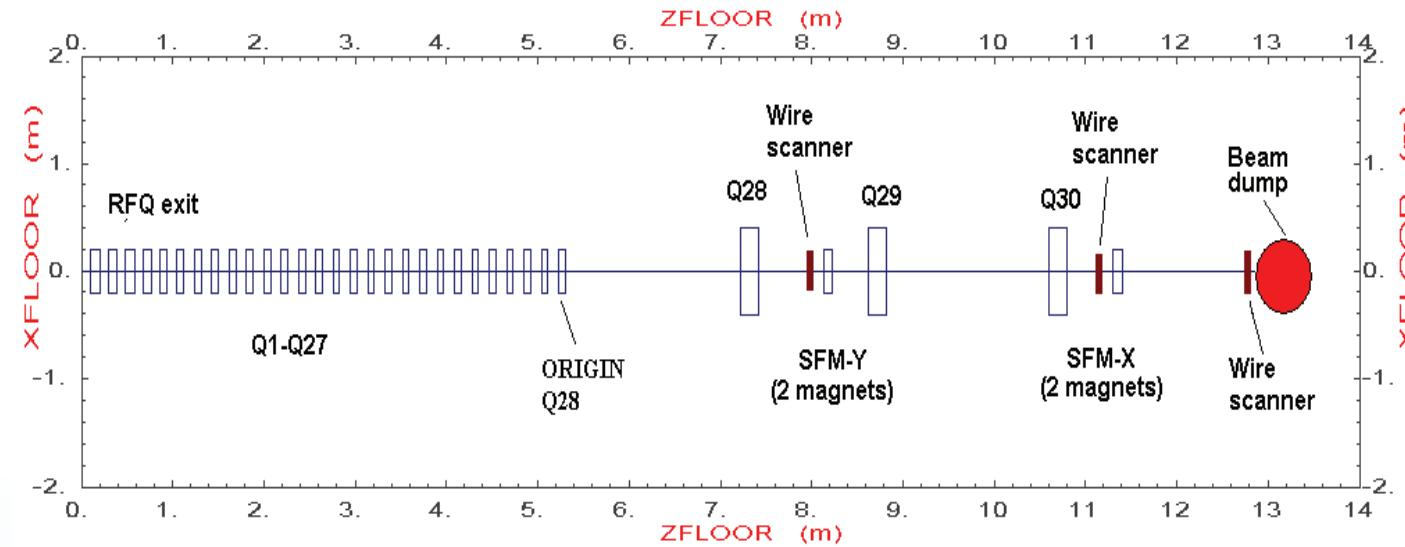
SFM can be step-like field magnets or simplified high-order magnets
