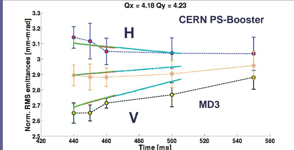
→ Accuracy of the RMS emittance measurements should be improved ...
