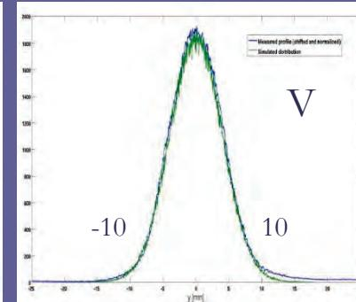
Generated and measured transverse beam profile at the 160MeV energy
