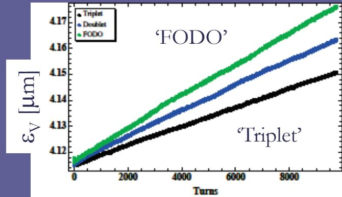
Variation of the beam size can lead to the emittance growth:
