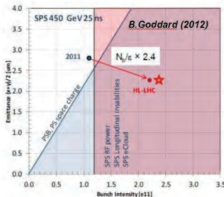
2011:  $\sim 1.1\text{e}11$  with  $2.8\mu\text{m}$  for 25nsec
