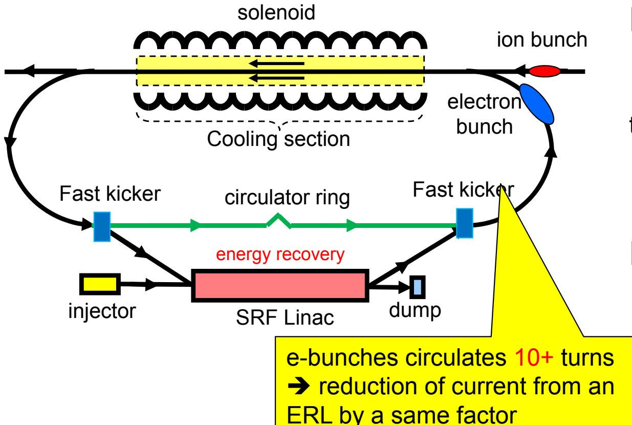
**Optimization:** Put it at center of the Figure-8 ring, for eliminating the long return path doubles the cooling rate
