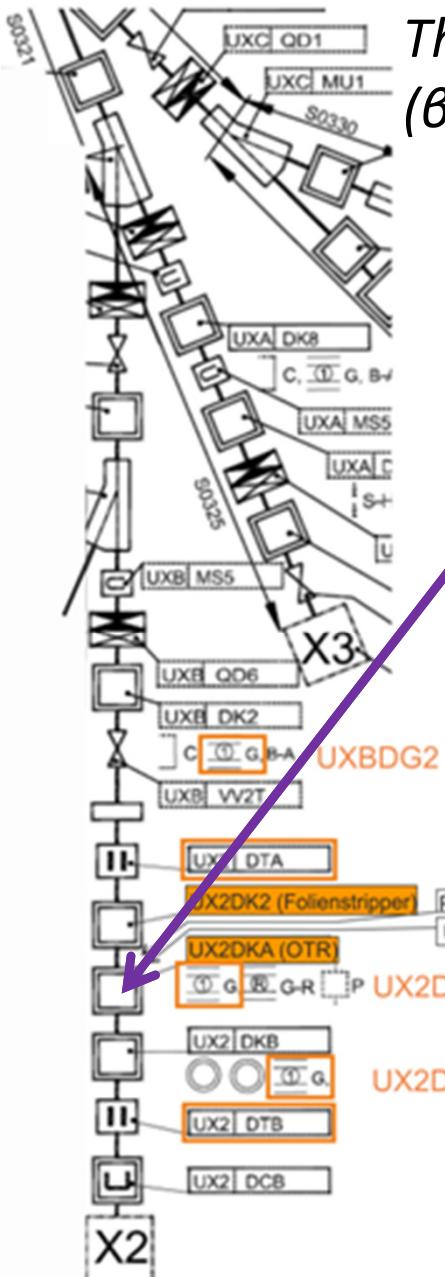
The feasibility of OTR has been evaluated with an 11.4 MeV/u ( $\beta=0.16$ )  $U^{28+}$  beam at the UNILAC (X2 beam line)
