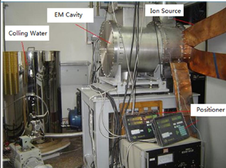
The ion source emittance is measured.
