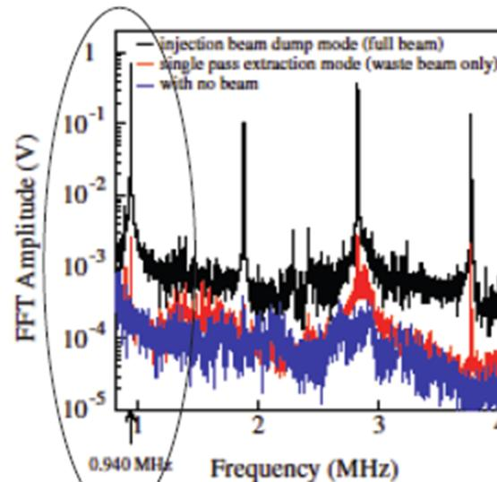
Typical waste beam signal measured by a CT
