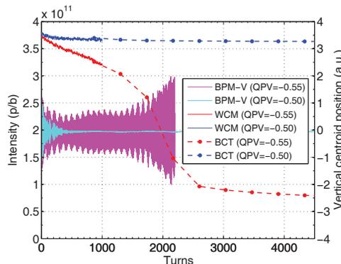
Figure 3: The intensity obtained from the wall current monitor (WCM) and the beam current transformer (BCT) are shown together with the vertical centroid position for two different settings for vertical chromaticity. Losses close to injection are due to injection oscillations.
