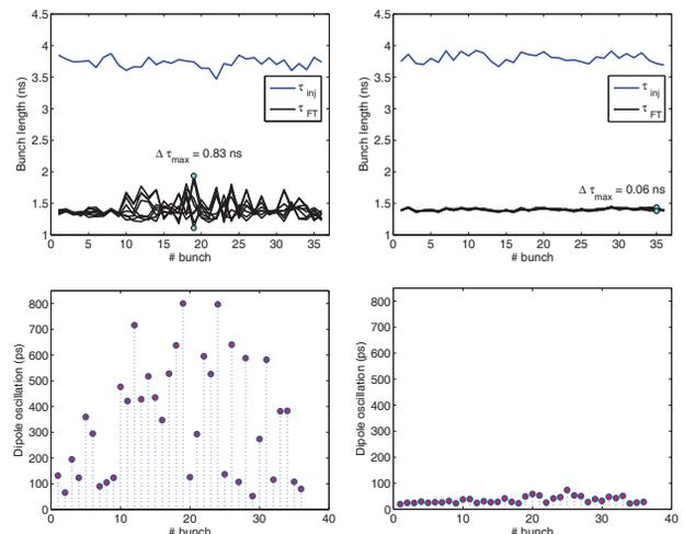
Figure 8: Bunch length (top) and bunch position (bottom) oscillations at flat top for the bunches of a single batch 50 ns LHC beam, for Q26 (left) and for Q20 (right).
