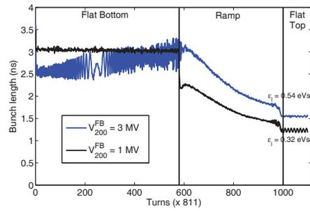
Figure 7: Bunch length evolution along the cycle for single bunches ( $N_b \approx 1.1 \times 10^{11}$  p/b) in Q26 with single RF system for two different capture voltages. The voltage programs after the flat bottom are the same in both cases.
