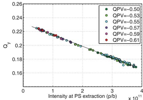
Figure 2: Vertical tune as function of intensity at PS extraction for different settings of the vertical chromaticity knob.
