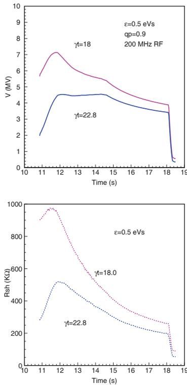
Figure 6: Voltage programs (top) and narrow-band impedance thresholds (bottom) through the cycle for Q26 (blue curve) and Q20 (magenta curve) optics in a single RF system for longitudinal emittance  $\varepsilon_l = 0.5$  eVs. Acceleration starts at 10.86 s.
