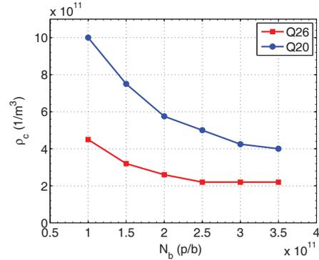
Figure 5: Threshold electron density  $\rho_c$  as function of the bunch intensity  $N_b$  for the nominal and the Q20 optics as obtained with HEADTAIL for injection energy.
