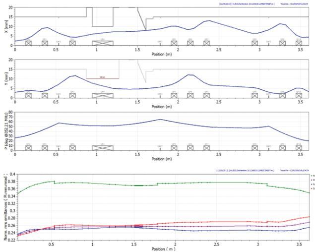
Figure 5: MEBT Layout and emittance evolution.
