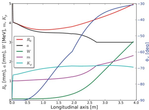
Figure 3: Main parameters evolution within the RFQ.
