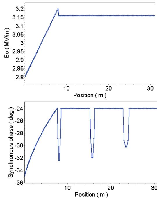
Figure 6: Design E0 and synchronous phase, along the DTL.
