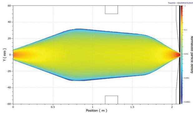
Figure 2: Beam density in the Y plane along the LEBT.
