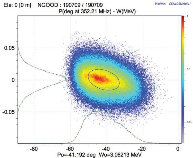
Figure 4: Longitudinal phase space at the RFQ exit.
