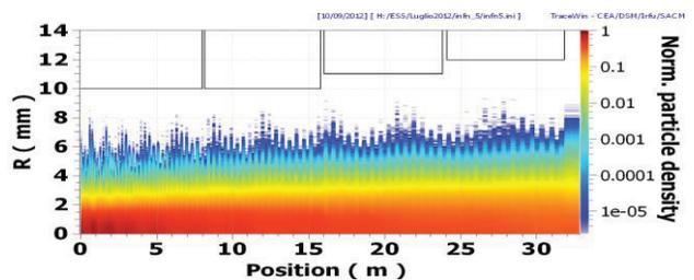
Figure 8: Particles density along the DTL.
