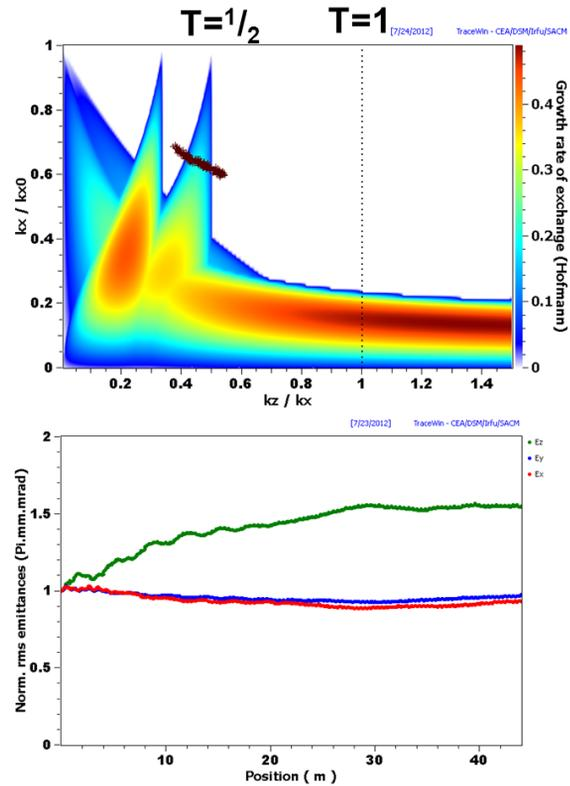
Figure 8: Chart and emittances for same case as in Fig. 6, but  $k_{x0}$  lowered to  $47^\circ$  ( $\epsilon_x$ : red,  $\epsilon_y$ : blue,  $\epsilon_z$ : green line).
