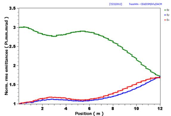
Figure 3: Chart (top) and emittance evolution (bottom) for crossing in 20 cells ( $\epsilon_x$ : red,  $\epsilon_y$ : blue,  $\epsilon_z$ : green line).
