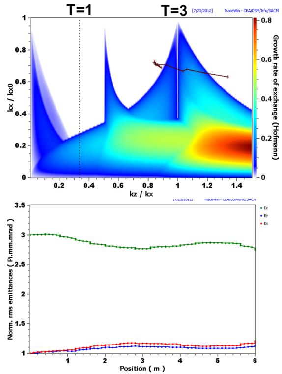
Figure 2: Top: Stability chart for  $\epsilon_z/\epsilon_x = 3$  and crossing over main resonance in 5 cells; bottom: evolution of emittances ( $\epsilon_x$ : red,  $\epsilon_y$ : blue,  $\epsilon_z$ : green line).
