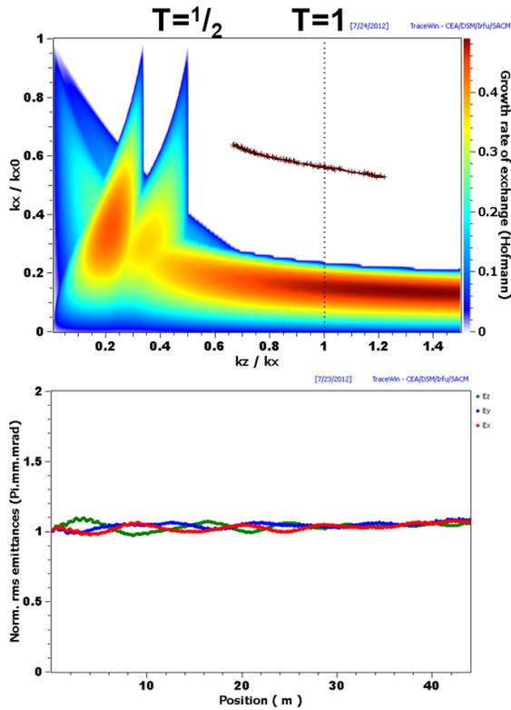
Figure 6: Chart for  $\epsilon_z/\epsilon_x = 1$  and emittance evolution for tune sweep from right to left over 100 cells ( $\epsilon_x$ : red,  $\epsilon_y$ : blue,  $\epsilon_z$ : green line).
