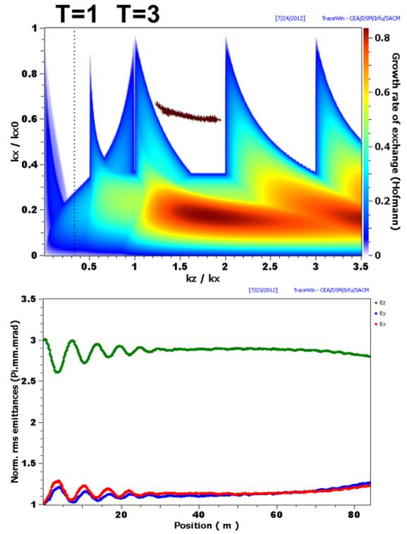
Figure 5: Chart and emittance evolution for tune crossing from left to right over 200 cells ( $\epsilon_x$ : red,  $\epsilon_y$ : blue,  $\epsilon_z$ : green line).
