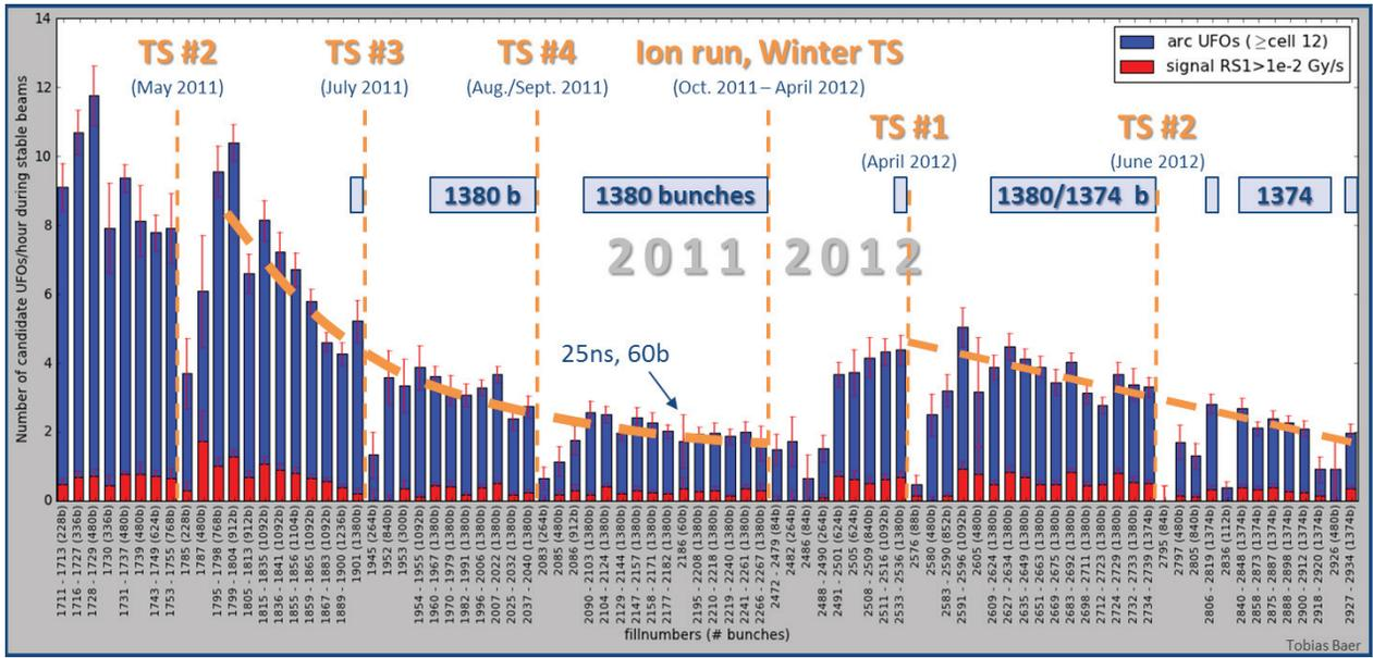
Figure 3: UFO rate evolution throughout the 2011 and 2012 runs. Only UFOs detected in the arc during fills of a duration larger than one hour are considered.
