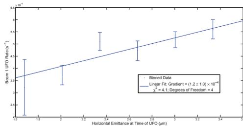
Figure 6: UFO rate vs normalized horizontal emittance calculated from BSRT beam size measurements at the moment of UFO occurrence. Only LHC fills from April until July 2012, with duration larger than 1 hour and 1374 or 1380 nominal bunches are considered.
