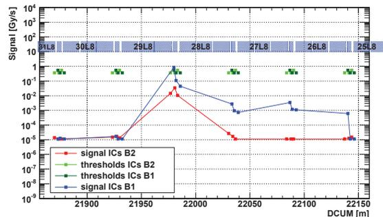
Figure 1: Longitudinal profile of a UFO in the LHC arc.
