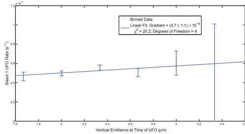
Figure 5: UFO rate vs normalized vertical emittance calculated from BSRT beam size measurements at the moment of UFO occurrence. Only LHC fills from April until July 2012, with duration larger than 1 hour and 1374 or 1380 nominal bunches are considered.
