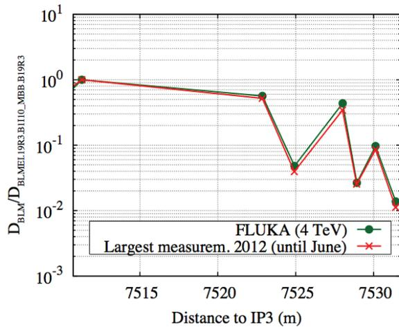
(b) Normalized signal for data and fluka simulation
