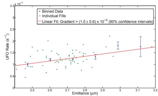
Figure 4: UFO rate vs normalized emittance calculated from luminosity at the beginning of the LHC fill. Only fills from April until July 2012, with duration larger than 1 hour and 1374 or 1380 nominal bunches are considered.
