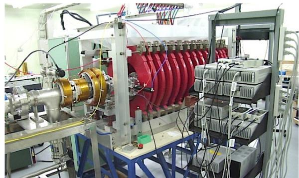
Figure 4: The Penning trap for S-POD IV.
