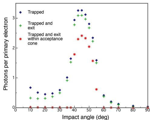
Figure 2: FLUKA estimates of the photon yields in a multimode Cherenkov fiber of diameter  $365 \mu\text{m}$  fiber with NA 0.22, as a function of the angle of an incoming charged particle with  $\beta=1$ .
