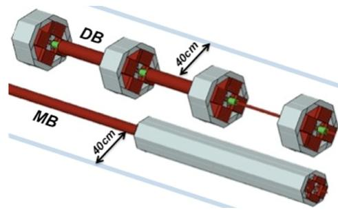
Figure 3: Representation of the two beam modules in FLUKA simulations.
