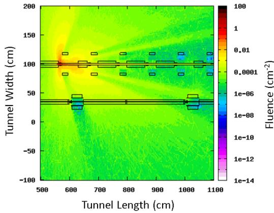
Figure 4: Spatial distribution of electron and positron fluences near the beam line resulting from a drive beam loss of 2.4 GeV, scaled to 1 lost electron.
