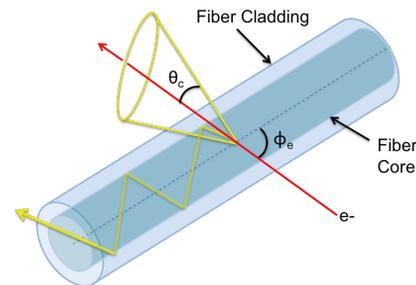
Figure 1: Schematic to illustrate the detection principle for Cherenkov beam loss monitors.
