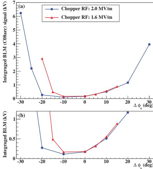
Figure 7: (a) The integrated BLM signals as a function of driving phase with respect to the angle with maximum deflection angle. The RF amplitude is set to 2.0 (blue) and 1.6 (red) MV/m. (b) Same as (a) but expansion of low beam loss region.
