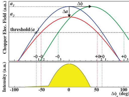
Figure 3: (Top) the chopper RF wave form at various conditions. (Bottom) Supposed beam distribution from the phase scan. The vertical axis is logarithmic scale.
