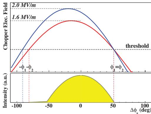
Figure 8: RF wave of 2.0 MV/m at  $\Delta\phi_s = -20$  deg (blue) and 1.6 MV/m at  $-15$  deg (red). Assuming the crossing-point is equivalent to the edge of the beam core in the positive phase side, we obtained half width to be 50 deg.
