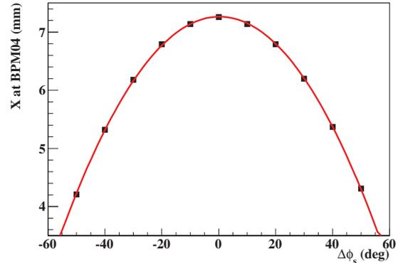
Figure 4: The correlation between the RF phase of the chopper and the beam position at Q1 in MEBT1. The horizontal axis shows the difference of the phase which is obtained by nominal tuning. The red line is the fitting result by quadratic function.
