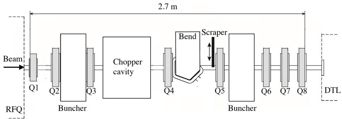
Figure 1: Layout of MEBT1. The RF chopper system, which is comprised from an RF chopper cavity and a scraper, is placed at the middle of MEBT1.
