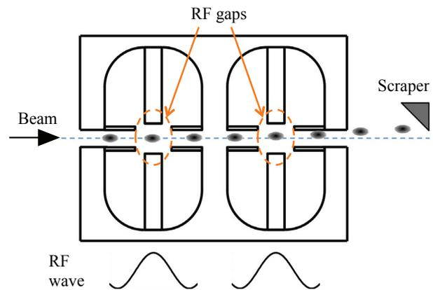
Figure 2: The outline of the chopper cavity. Two RF gaps are in the cavity for the horizontal deflection. The deflected beam is absorbed in the scraper. The RF phase is adjusted as the beam is deflected at an RF peak.
