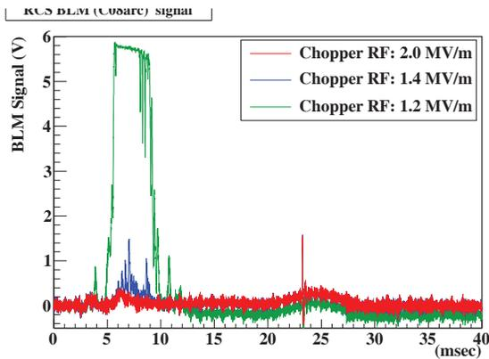
Figure 5: Time evolution of the BLM (C08arc) signal for one acceleration cycle of RCS. The acceleration starts soon after the beam injection at 3 msec, and then the beam is extracted at 23 msec. The signal distributions at the RF amplitude of 2.0 (red), 1.4 (blue) and 1.2 MV/m (green) are plotted. We integrate the BLM signal from 3 to 12 msec for the evaluation of beam loss.
