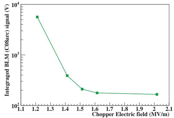
Figure 6: The integrated BLM signal as a function of chopper RF amplitude. The driving phase of the chopper is adjusted at the maximum deflection angle.
