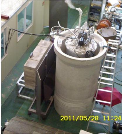
Figure 12: Experiment of the PEFP SRF cavity.
