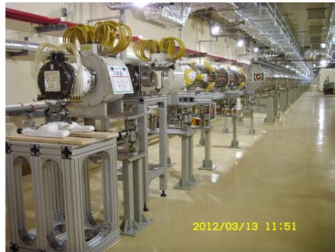
Figure 6: PEFP 100-MeV linac installed into the accelerator tunnel.
