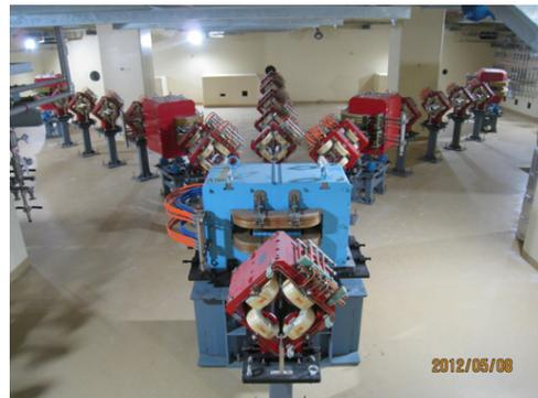
Figure 7: The beam line magnets installed for 20-MeV beam line.
