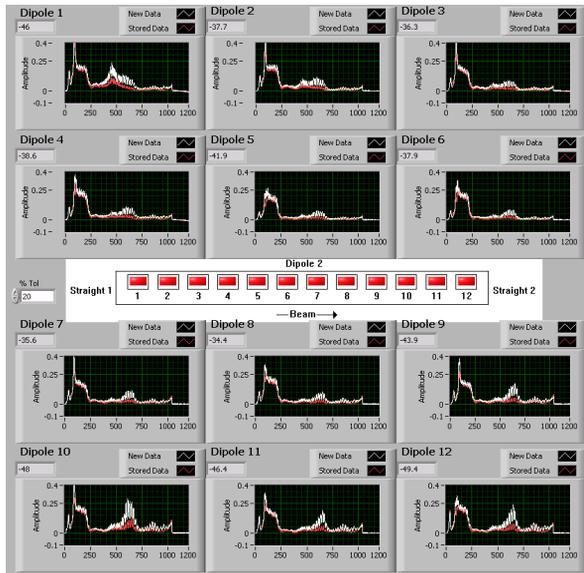
Figure 8: Ring dipole 2 scintillator outputs showing large mid cycle beam loss (white), previous reference (red).
