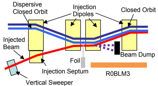
Figure 4: Schematic layout of the injection system.
