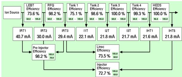
Figure 2: MCR Screen:Injector intensity monitor efficiencies.
