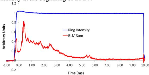
Figure 6: Sum BLM and intensity versus acceleration time.
