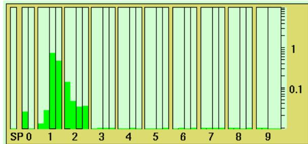
Figure 7: MCR Screen: Integrated ring beam loss (Vs) on each BLM over the acceleration cycle, 0-10 ms.
