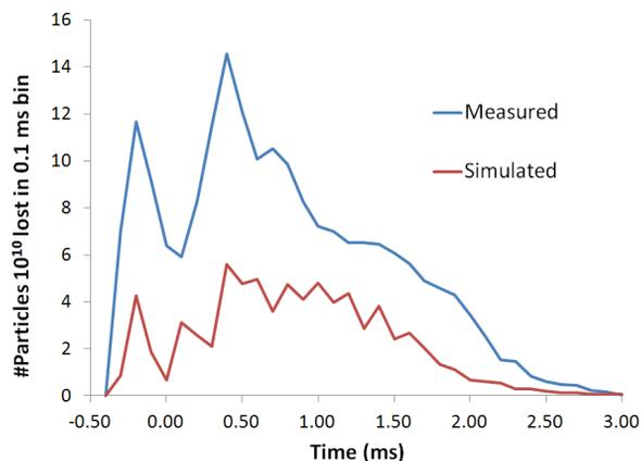
Figure 11: Measured versus predicted beam loss.
