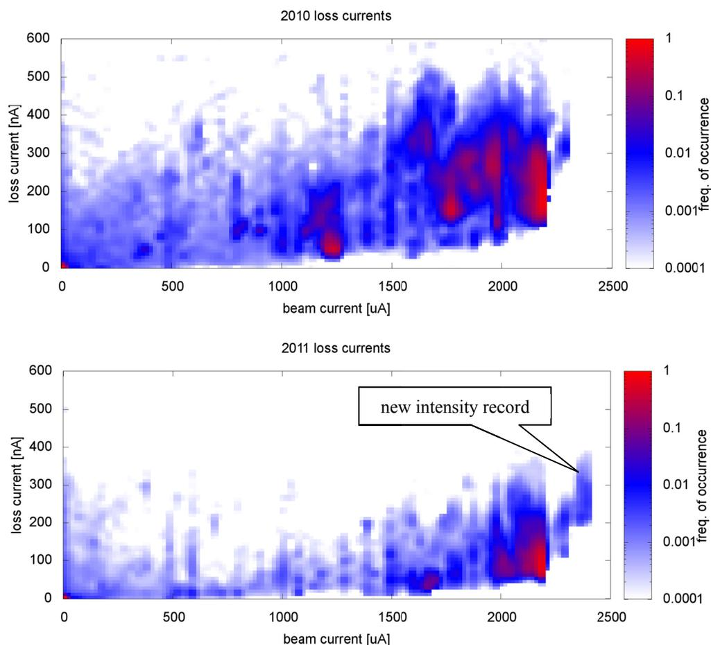
Figure 5: Beam losses as a function of beam current for the years 2010 and 2011. The color code corresponds to the frequency of operation at a certain combination of loss current and beam current. Note the logarithmic scale of the color code.
