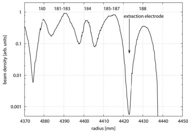
Figure 4: Beam density measured at extraction on a logarithmic scale. The turn numbers are indicated at the peaks.
