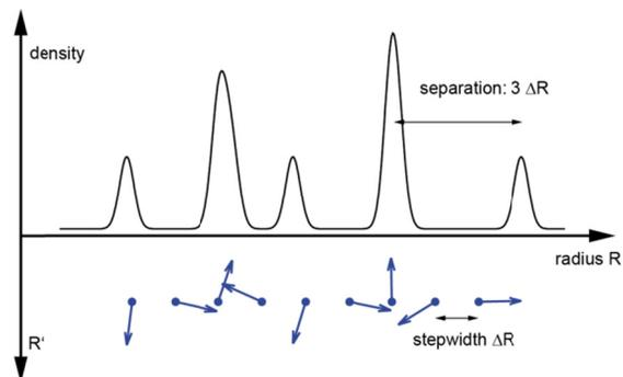
Figure 3: Using eccentric injection, the turn separation at the extraction septum can be maximized. The figure shows radial phase space vectors of the orbit oscillations and the resulting beam density.
