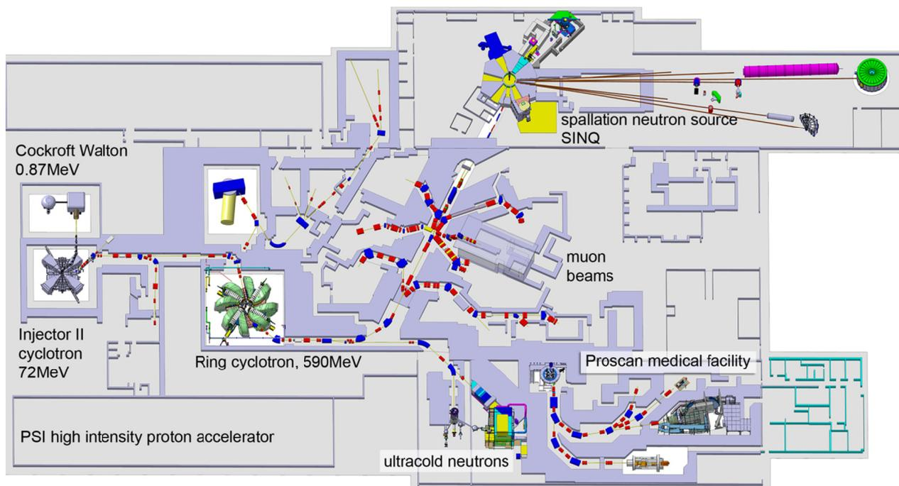
Figure 1: Layout of the PSI high intensity proton accelerator including the two meson production targets (center of image) and the spallation neutron source SINQ with related experimental facilities. The proton therapy facility for cancer treatment was originally connected to HIPA, but uses a separate superconducting cyclotron now.
