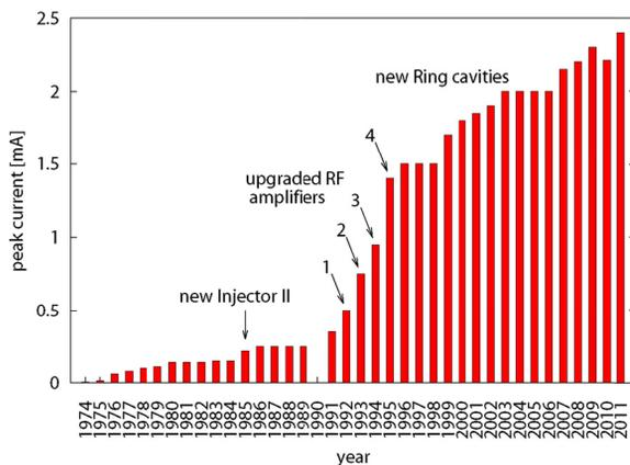
Figure 2: Development of the maximum attainable beam current in the HIPA facility.
