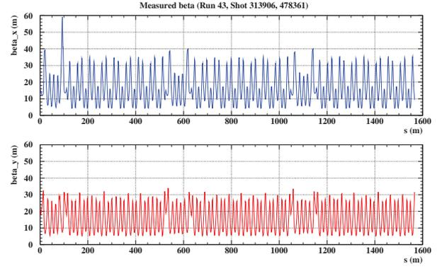
Figure 2: Measured beta function.
