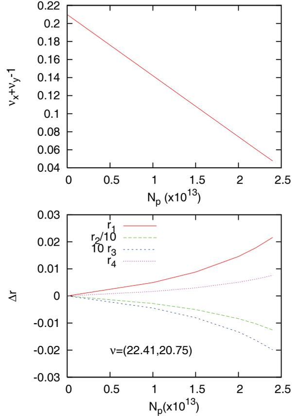
Figure 4: (Preliminary) Tune summation (top) and x-y coupling parameters (bottom) given by solving the beam envelope equation.
