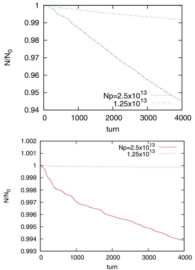
Figure 6: (Preliminary) Intensity dependence of the beam loss. Top picture is obtained for  $V = B_{mes}R_{mes}$ . at both of space charge and sextupoles. Bottom picture is obtained for  $V = B_{mes}R_{mes}$ . at space charge and  $V = B_0R_0$  at sextupoles.
