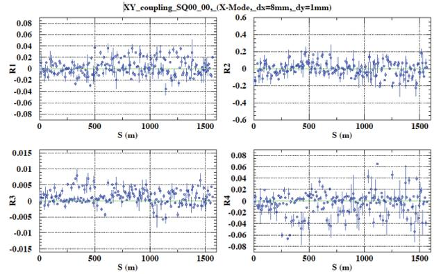
Figure 3: Measured xy coupling parameters.
