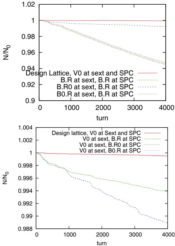
Figure 5: (Preliminary) Beam loss for various cases of  $V$  given by simulation.
