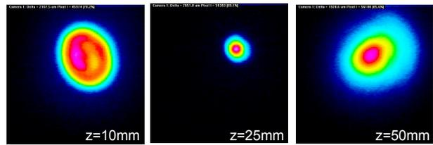
Figure 3: Laser modes measured along a beam path before and after a focusing lens. These were used to extract profiles in x- and y for the M<sup>2</sup> calculation.
