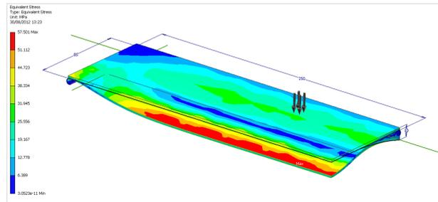
Figure 9: Example of static pressure simulation to check the stability of bottom and lid. The shown example tapers from just 2 mm around the central path up to 10 mm near the side walls.
