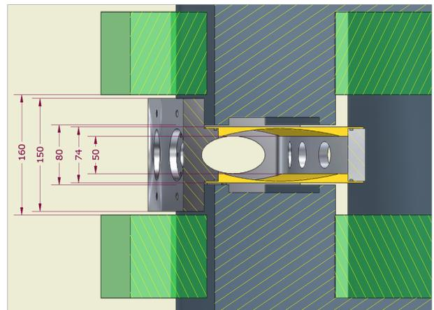
Figure 8: Both vessel and magnet shown. The coils provide the space for the flanges of the three beam lets and the movables stage to scan the laser. Due to tapering towards the centre a minimal clearance of at least 40–45 mm is sustained everywhere.
