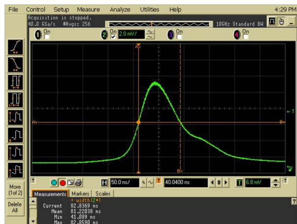
Figure 4: Temporal behaviour of the laser pulse, measured with a 50 ps photo diode and a 50 Gs/s, 10 GHz oscilloscope. Top, the PA is triggered with a 3 KHz signal, shown green is the 30 kHz pulse of the MO. Below, such a single pulse is resolved in time,  $\tau=83$  ns at FWHM.
