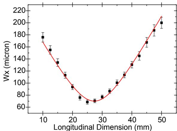
Figure 5: Fitted envelope to beam radii in near and far field at clip points of 13.5%. Each radius was averaged over 64 measurements. For the x-plane  $M^2=1.61$  and for the y-plane it is  $M^2=1.81$
