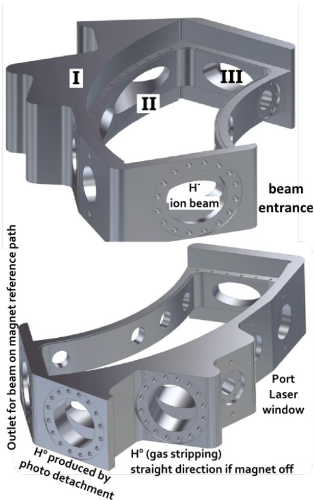
Figure 6: Two different views of the vessel design. The narrower part fits in between the magnet yokes. The side walls are higher to provide space for flanges mounted without adapters to save space. The coils need to be provide vertical clearance that the side wall fits in between.
