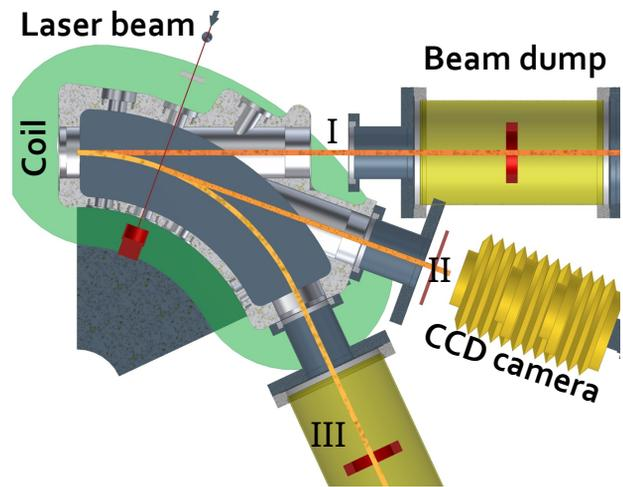
Figure 7: Impression of the whole assembly with all three beam lines. Despite all the effort to provide enough space for the neutrals (2<sup>nd</sup> beamlet) the space for scintillator and camera is tight due to the radial dimensions of the beam dump (at least CF250).
