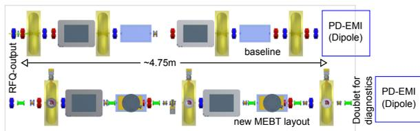
Figure 2: Above, the standard MEBT layout with 4 bunchers and 11 quadrupoles is shown (baseline-design). Below, a very new proposal is which is longer yet less elements. More drift space can be used for e.g. diagnostics or vacuum. There is the possibility of reduced costs for the new proposal. But at least one more doublet is required to focus the beam into the diagnostics.
