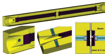
Figure 1: A view of a single jaw and cross-sections of the mock-up collimator with in-jaw BPM buttons [10].
