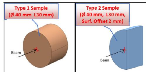
Figures 8-9: Type 1 (left) and type 2 (right) material sample shapes.
