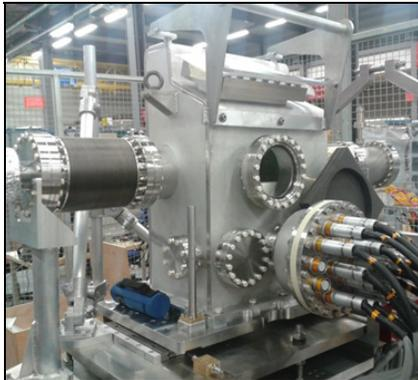
Figure 12: Stainless steel vacuum tank.
