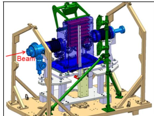
Figure 7: General assembly of the sample holder.
