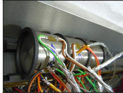
Figure 13: Strain gauges mounted on Inernet® specimens.
