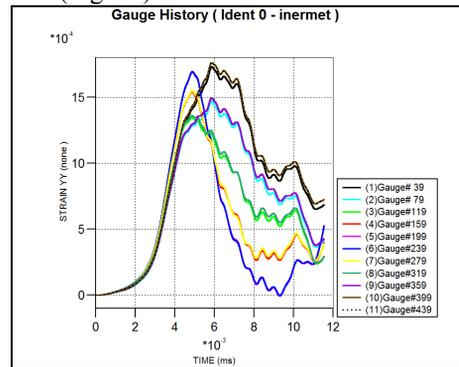
Figure 14: Expected circumferential strain in different axial positions for Inernet®, 440GeV energy, 3e12 protons/pulse.
