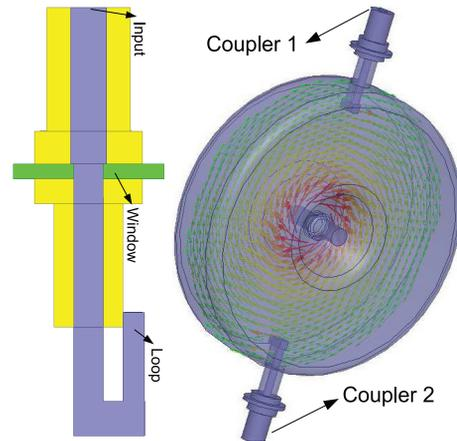
Figure 6: **Left:** Electromagnetic model of the drum-like coupler including the coupling loop designed for the cavity. **Right:** Magnetic field intensity  $H_\theta$  of the  $TM_{010}$  mode resonating in the cavity induced by the power couplers.
