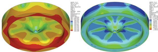
Figure 7: Ansys temperature (left) and stress (right) fields.
