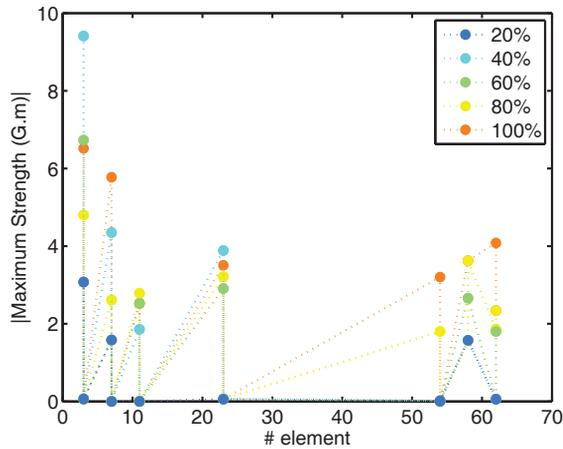
Figure 4: Maximum strength (|G.m|) obtained for each steerer, considering the proposed layout. Results are presented in steps, going from 20% error, 40%, upto 100%.
