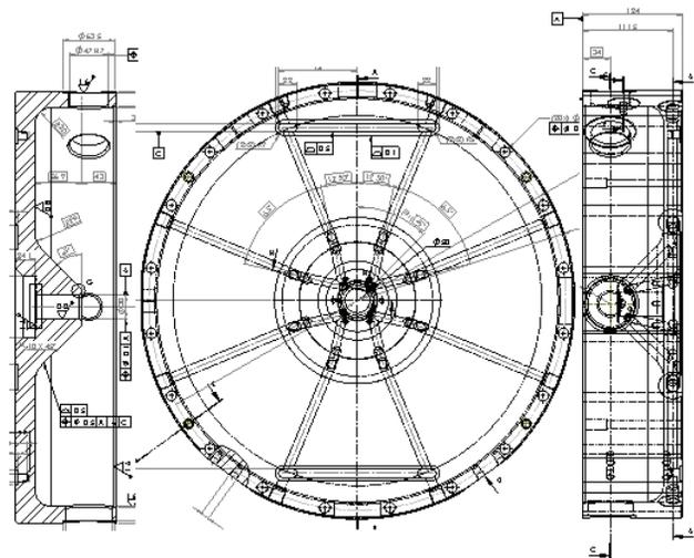
Figure 8: Engineering detail of the A30W126T45v1 buncher cavity drawings with its characteristic Maltese cross shape cooling channels.
