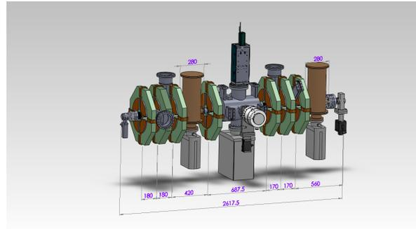
Figure 1: Mechanical layout of the MEBT1.
