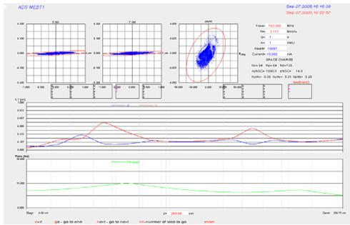
Figure 3: RMS beam envelope in MEBT1 by Track.
