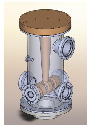
Figure 6: Room temperature(r.t.) QWR buncher cavity.
