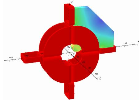
Figure 5: Quadrupole with steering coils.
