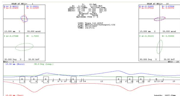
Figure 2: Beam envelopes in MEBT1 by Trace3D.
