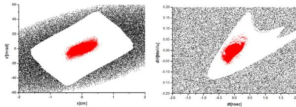
Figure 4: Acceptance(white margin) and emittance(red solid) at MEBT1 exit. Left: transverse phase space. Right: longitudinal phase space.
