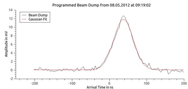
Figure 4: Beam losses due to a beam dump measured with 20 dB amplification. It is a typically Gaussian loss profile with a standard deviation of 52 ns.
