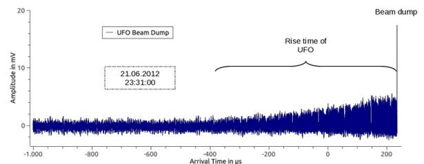
Figure 8a: Diamond measurement of beam losses due to an UFO event from the 21.06.2012 at 23:31. The diamond signal is amplified by 20dB. The UFO has a rise time of  $\sim 600 \mu\text{s}$ .
