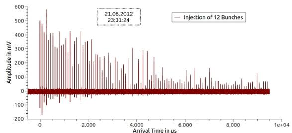
Figure 1a: Measurement of beam losses during injection of 12 bunches for beam 1 into the LHC. Signal amplification: 40 dB. The injection process leads to beam losses during 10 ms ( $\sim 110$  turns) and is decreasing after some turns.
