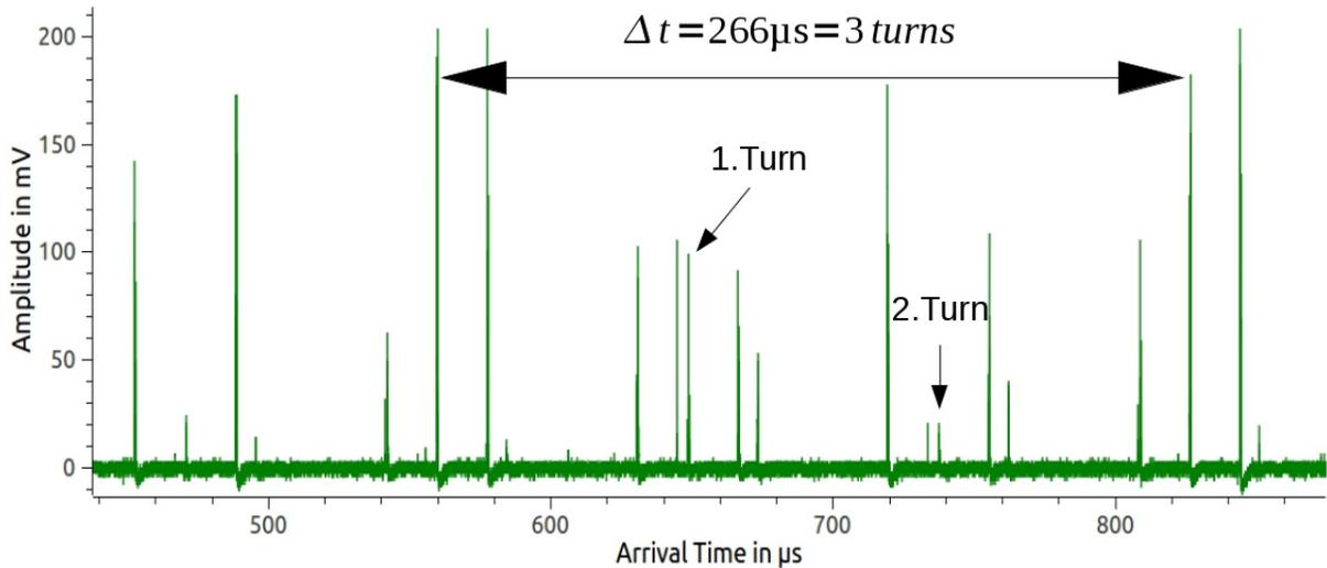
Figure 5a: Measurement from 29.05.2012 at 15:42 of beam losses caused by an instability in beam 1. Due to the fractional tune of  $\sim 0.3$ , the loss amplitude is modulated with a periodicity of 3 turns. Within 2 s several acquisitions were triggered. Signal amplification: 20 dB.
