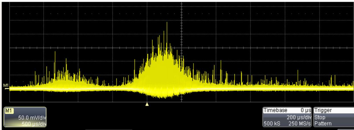
Figure 7: Gaussian beam loss profile as a function of time of two UFO events that occurred at the IR2 injection kicker magnets (beam 1) on the 20.08.2012 at 18:07. The signal of the IR7 diamond BLM is amplified by 40 dB.
