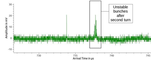
Figure 5e: Zoom of beam losses of unstable bunches after the second turn. The bunches have only small beam losses compared to the third turn.
