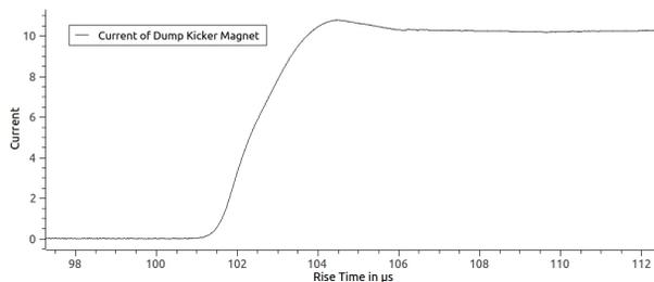
Figure 2: Rise time of a MKD. The rise time of the current during  $\sim 101 \mu\text{s}$  and  $\sim 104 \mu\text{s}$  is synchronized with the abort gap of the beam. After  $\sim 104 \mu\text{s}$  the MKD extracts the protons to the beam dump absorbers via the transfer-lines.
