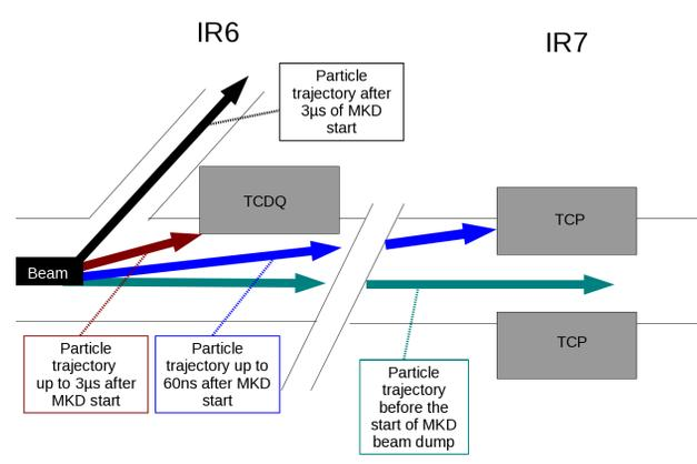
Figure 3: Illustration of particle trajectories during the rise time of the dump kicker. Unbunched protons in the abort gap are deflected and are mainly lost at the collimators in the beam dump (IR6) or cleaning region (IR7) due to the rise time of the kicker magnet.
