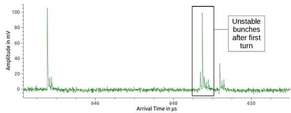
Figure 5d: Zoom of unstable bunches after the first turn. The beam losses are less due to a change of the phase advance.
