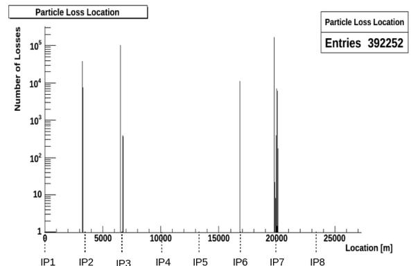
Figure 6: Simulated beam losses due to an UFO event at the injection kicker (IR2). Losses around the LHC ring at the collimators in IR2, IR3, IR6 and IR7 can be observed.
