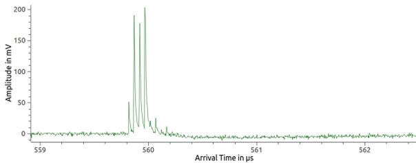
Figure 5b: Zoom of unstable bunches at an arrival time of  $\sim 560 \mu\text{s}$ . Only six bunches, that are separated by  $50 \text{ ns}$ , contribute to the beam losses.
