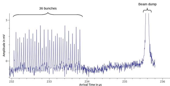
Figure 8c: Zoom into the very last bunches with beam losses right before the beam dump. The bunches are spaced by 50 ns and have different amplitudes due to the time resolution of 2 ns instead of 1 ns.
