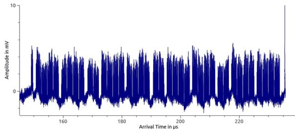
Figure 8b: Zoom into the last beam losses before the beam dump. The injection bunch pattern from the LHC is visible.
