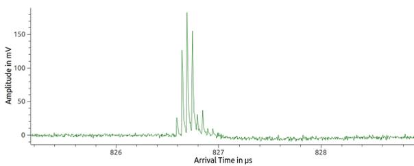
Figure 5c: Zoom of the same six bunches as in Fig. 5b but after the three LHC turns. The loss pattern is still the same.
