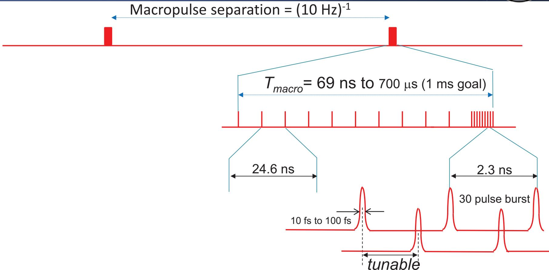
We plan on using an optical split and delay to generate sub-ns pulse separation
