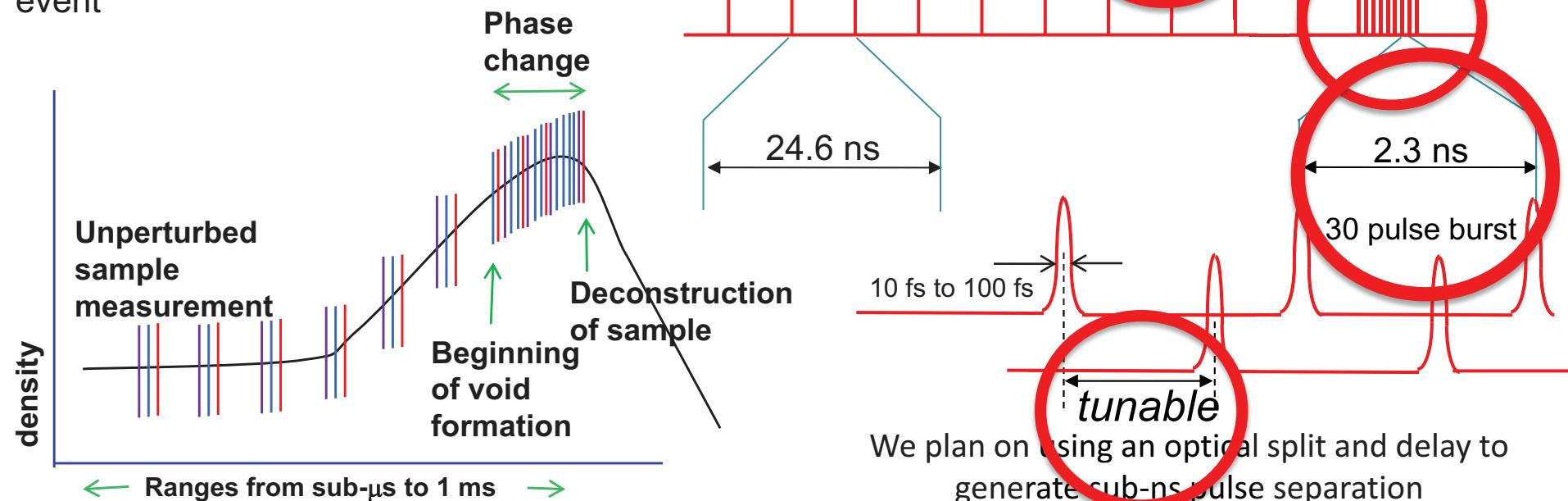
We plan on using an optical split and delay to generate sub-ns pulse separation
