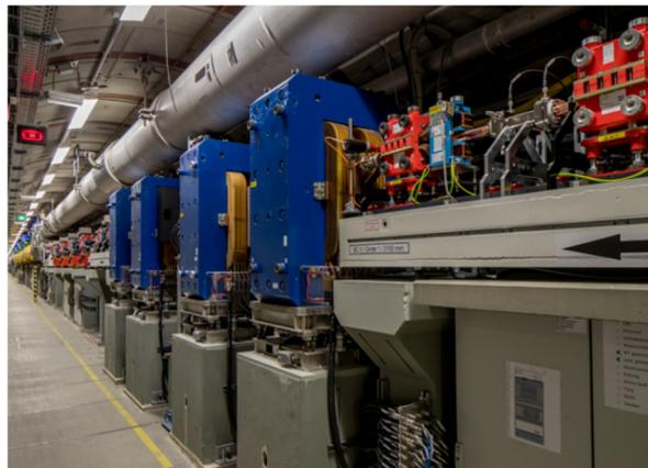
Figure 1: First bunch compression chicane.
